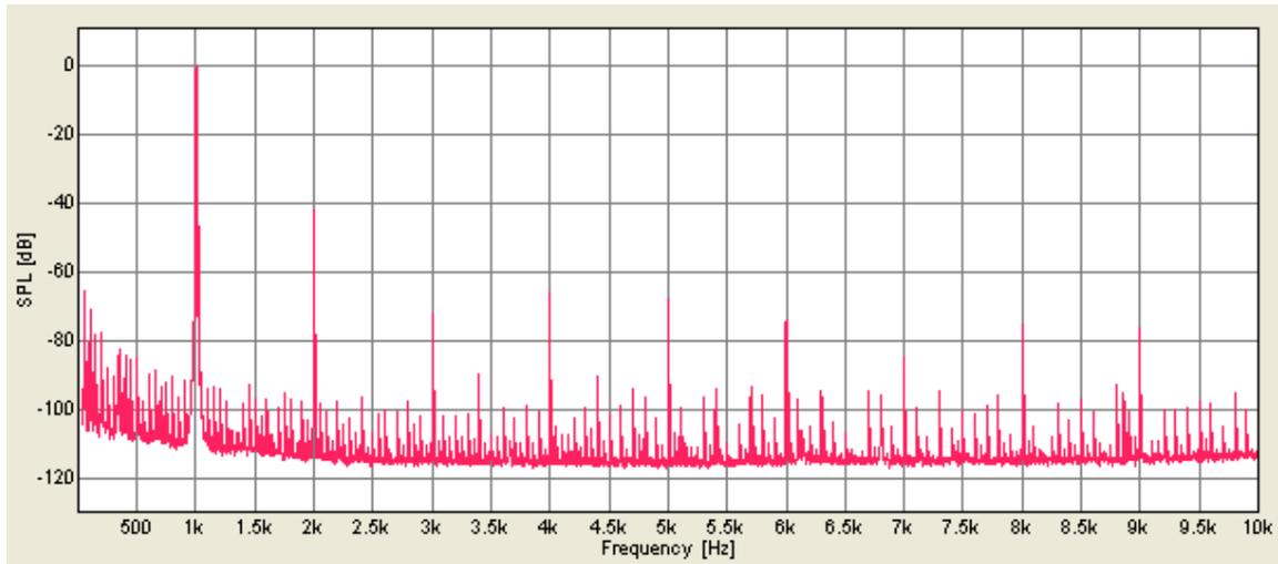
Figure 2: Harmonic distortion @ 1kHz and 0dBFS
