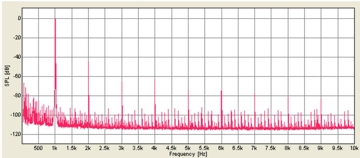
Figure 3: Harmonic distortion @ 1kHz and 0dBFS with somewhat lowered negative supply impedance
