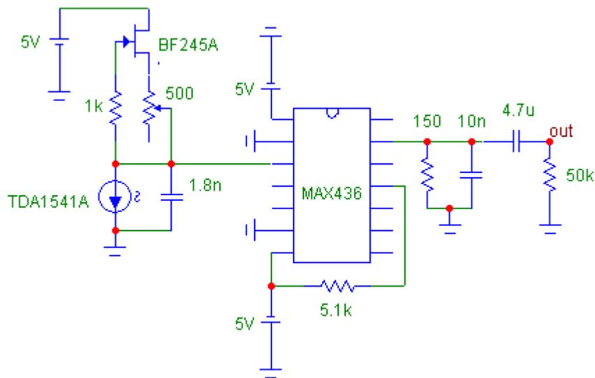
Figure 1: MAX436 applied for use with TDA1541A
